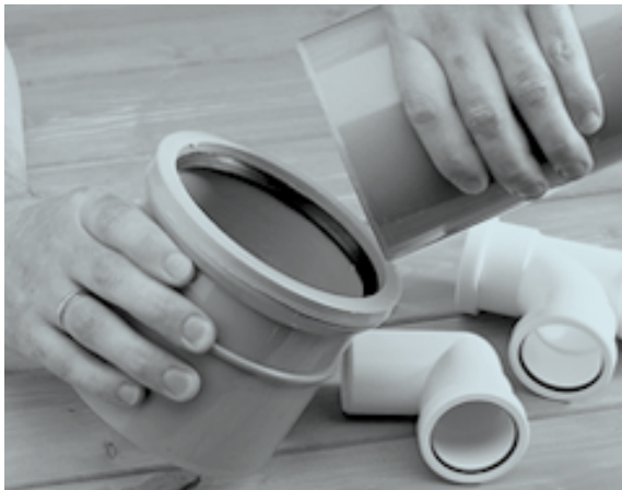
Push-fit (ring seal) assembly
